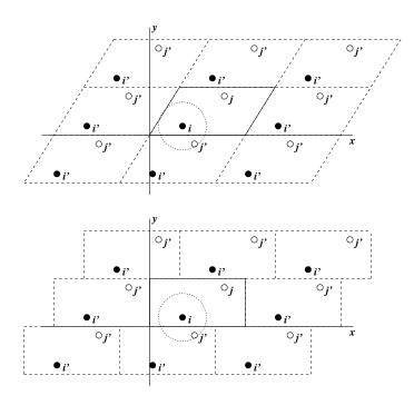
Fig. 5.1: Periodic boundary conditions in two dimensions.
