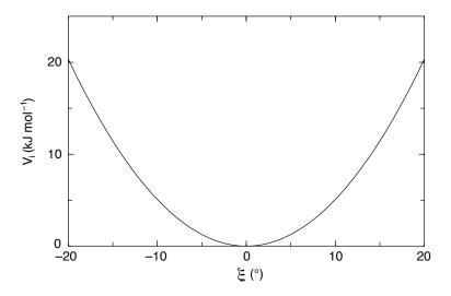
Fig. 5.25: Improper dihedral potential.
