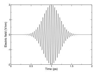
Fig. 5.48: A simulated laser pulse in GROMACS.
